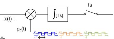
Encode the input signal by mixing with random code sequence (like spread spectrum)
