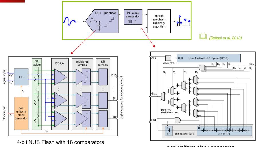
non-uniform clock generator with configurable under-sampling factor
