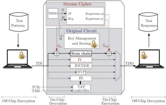
Mode of operations in 2 phases: initialization and encryption
