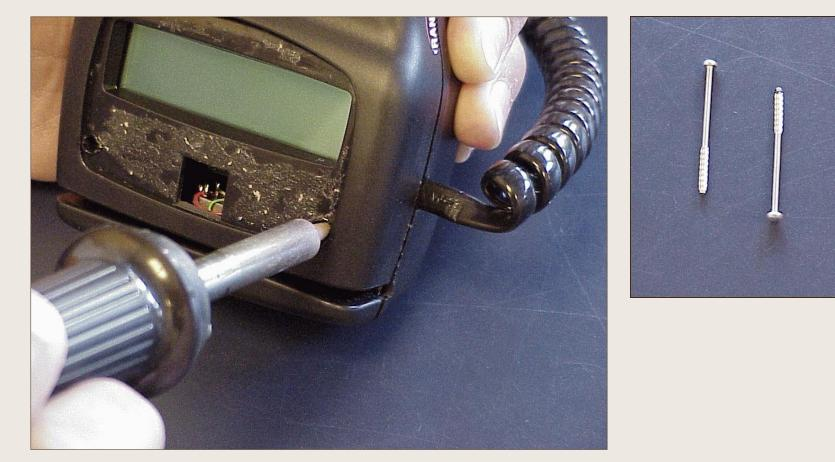
Removal of one-way screws via the front
